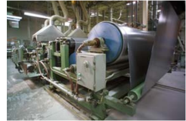
The recycled material being reprocessed into new membrane.
